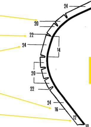
Fig. 2 shows a cut of the new glove along the lines II-II of Fig. 1, with the finger in its bent state:
