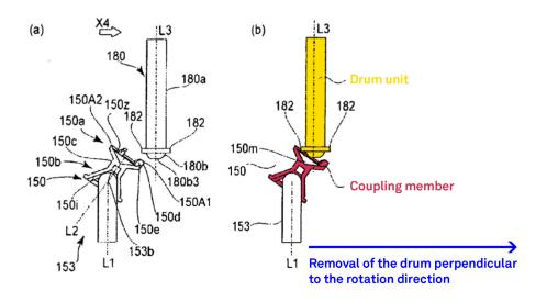
Ill. 1: Excerpt from Fig. 22 of the patent-in-suit (coloring and text added)
